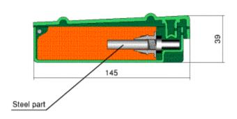
Length: 145 mm Width: 68 mm Height: 39 mm Mass: 400 g **Explosive charge:** 200 g TNT Body: Plastic Colour: Olive-drab Chemical Fuse type: Mode of activation: Pressure Sensitivity: 3 - 18 kps
