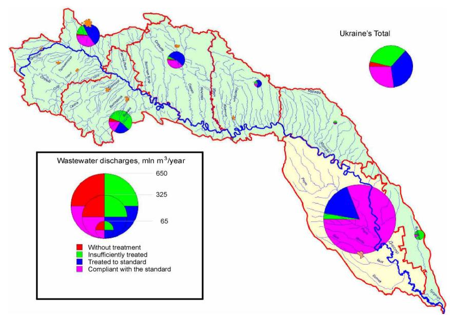
**Figure 3.6.** Wastewater Discharges in the Dniester Basin in 2002
