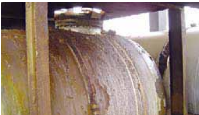
Leaking Melange Container, Kazakhstan, 2006
